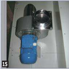
15 Air cooling extractor
