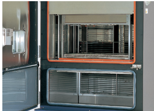
TSD Test areas ( Top: hot chamber Bottom: cold chamber )
